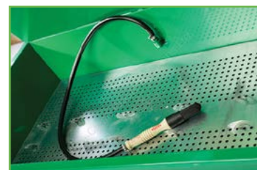
Handy flow through brush attached to solvent resistant hose for cleaning large parts.
