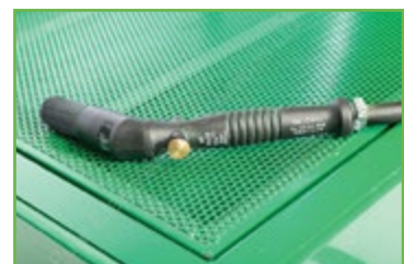
Flow through brush can be controlled by push button to assist flow control during cleaning of parts.
